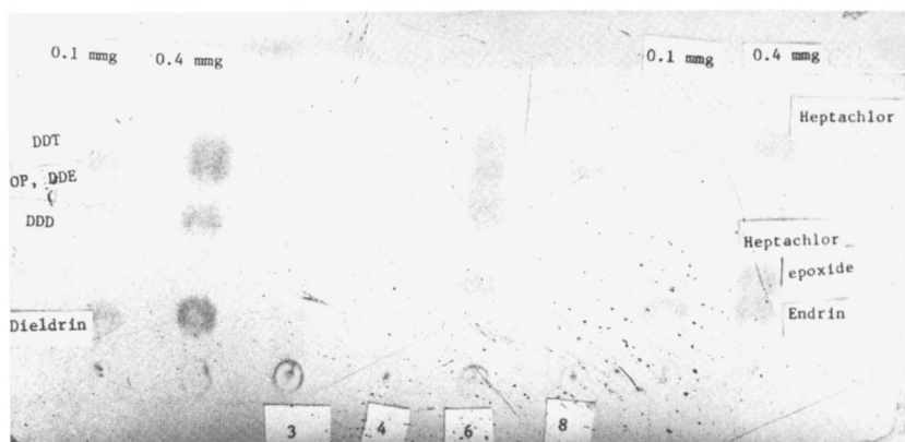
Figure 4. Thin-layer chromatogram of actual organochlorine residues in nursery soils
